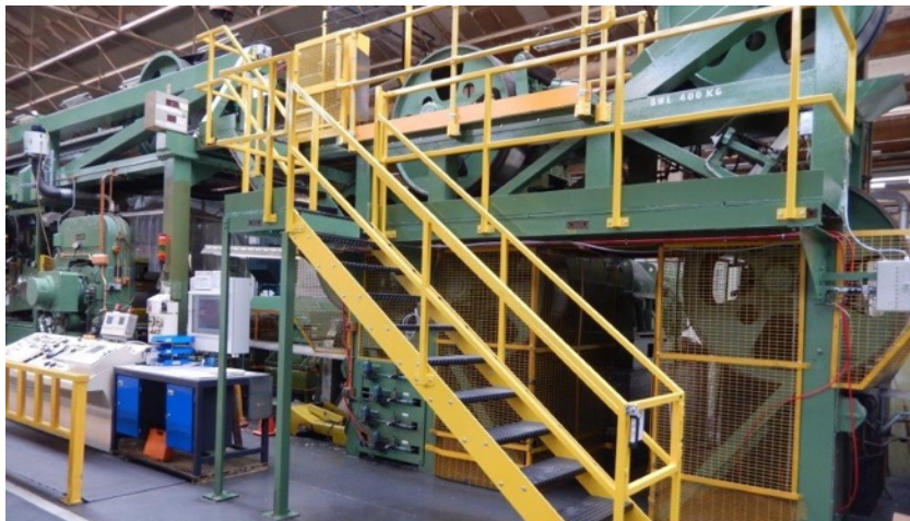
Staircase with handrails that meet the required standard height
