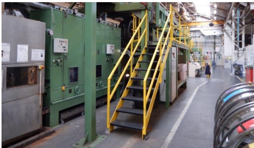
Staircase to access platform designed by Procter fits the plant space
