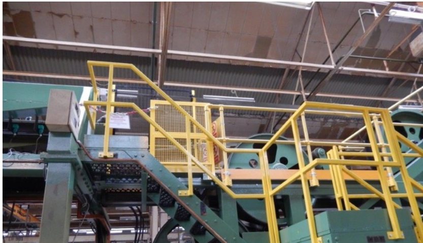
Access platform & stairs with handrails all made & installed by Procter
